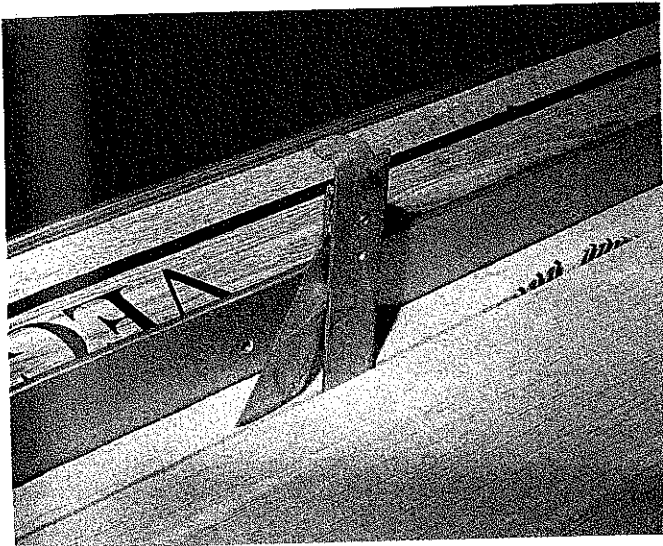
Fig. 6-16. Use the splitter when ripping stock.
